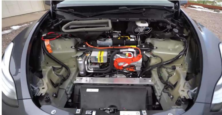
Figure 68. Tesla Y thermal management system [23].
