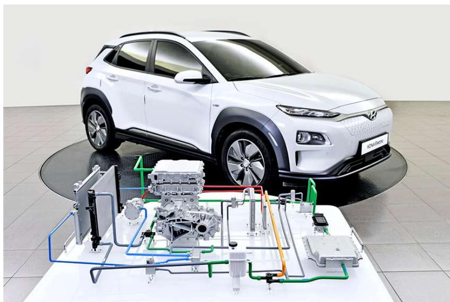
Figure 67 Photo Hyundai Kona EN and 3D of its heat pump system [22].
