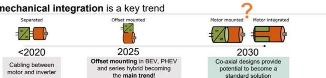
Figure 13 Different electro-mechanical integrations [9].
