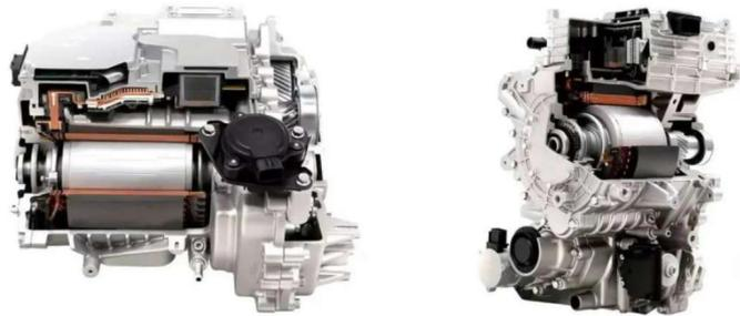
Figure 5. IONIQ 5 Hyundai front (left) and rear (right) drives assembly [3].
